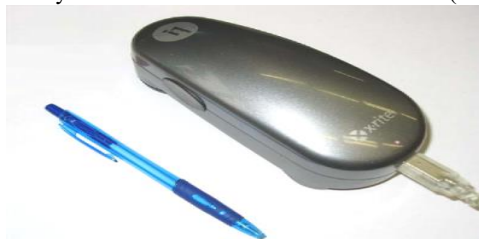
6-rasm. Eye-One Pro mini-spektrofotometer
