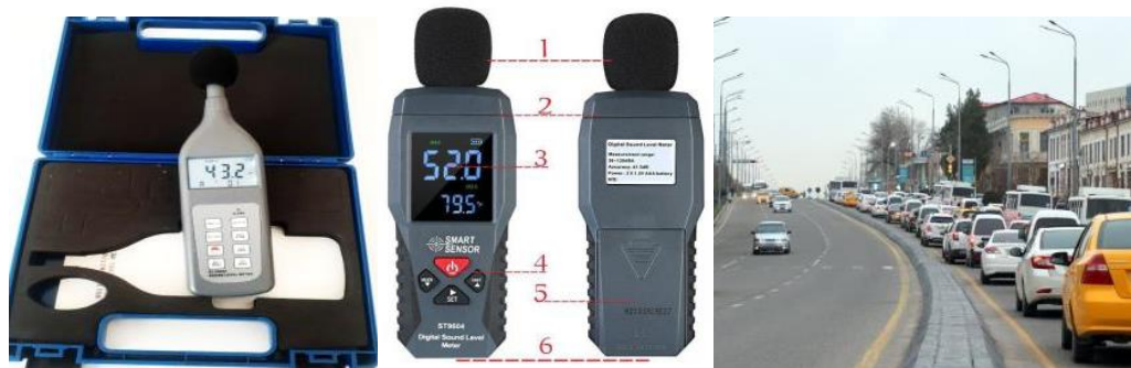
2-rasm. Sound Level Meter SL-5868P (shovqin o'lchagich) asbobining tuzilishi.
